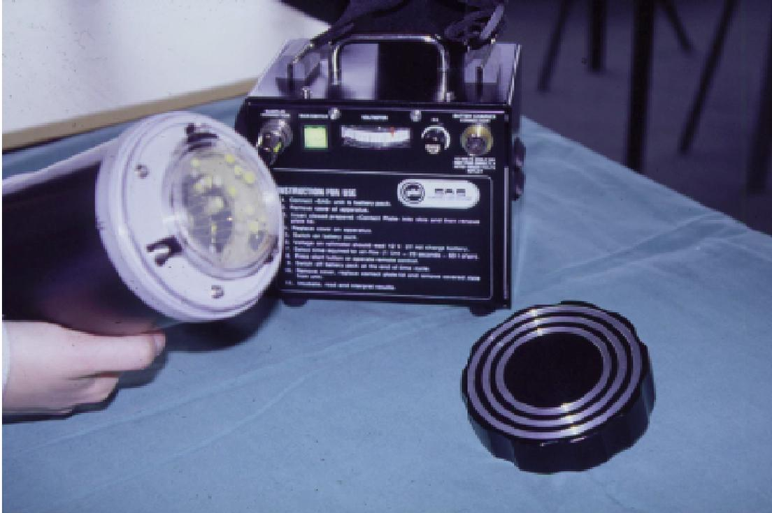
Figure 1. Surface Air Sampler (Cherwell Laboratories, Bicester, UK).
